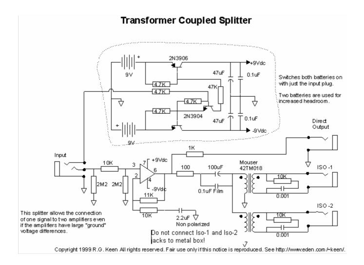
A transformer isolated signal splitter that enables hum-free connection of one guitar to more than one amp as well as having a direct output. The circuit is buffered to avoid signal loss.
